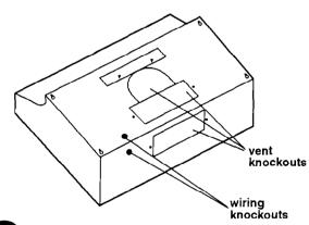
■ Remove knockout from the wiring ig (top or rear) to be used. For rectangular venting, remove only the 3-1/4" x 10" rectangular opening knockout.
